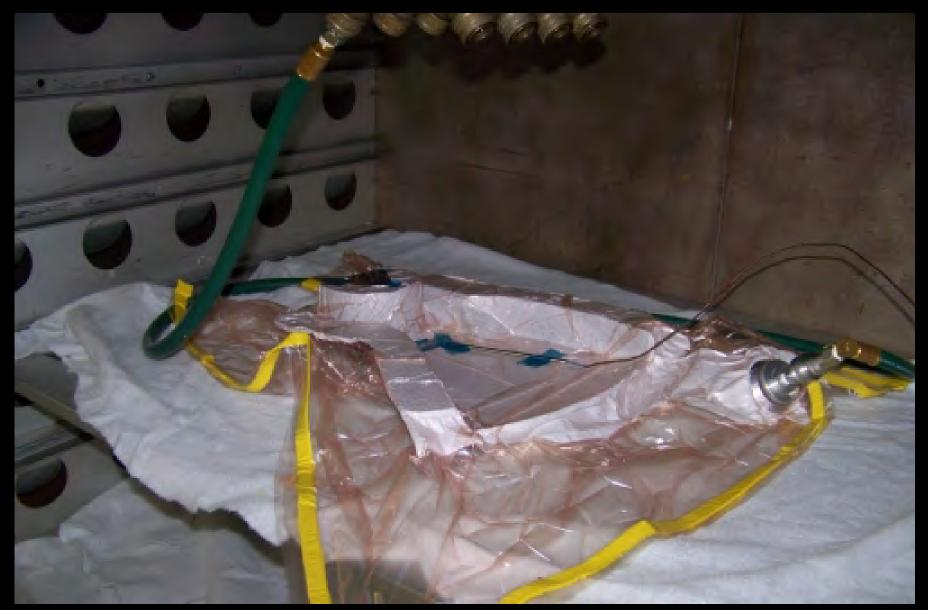
Use thermocouple that measures the temperature at the tool and not in the air. Following the prepreg manufactures cure cycle is important to achieving a high quality surface smoothness.
