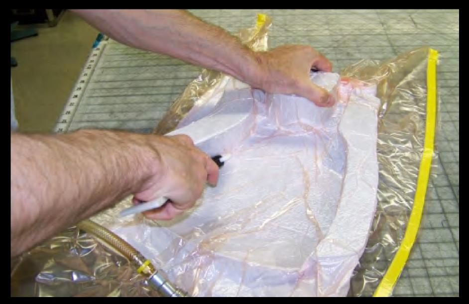
Ensure that the bag is not bridging at any corners, be careful not to cause a tear or puncture of the bag.
