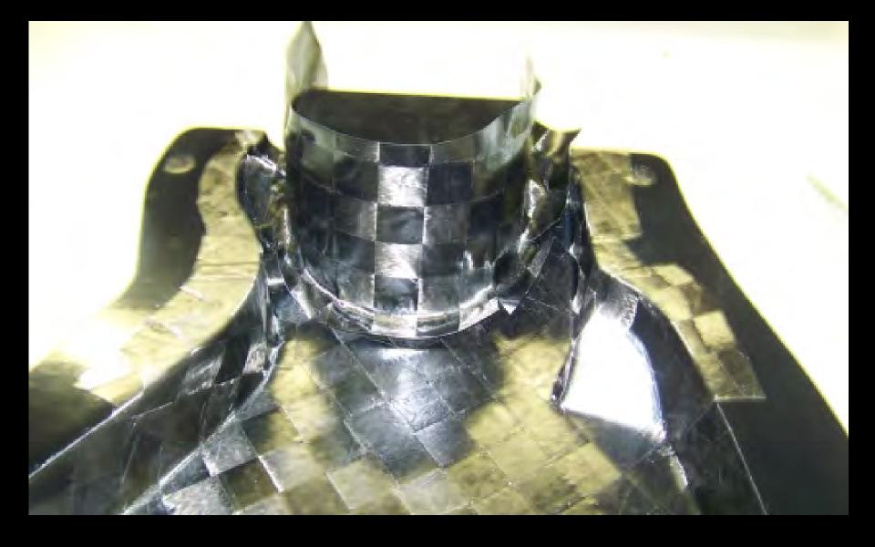
Start 2<sup>nd</sup> ply using the same sequence as the first, making darts where needed.
