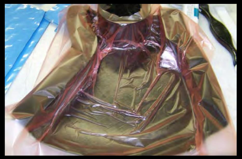
**Always debulk the first ply!** Perforated release film is recommended during this step due to the dense nature of TeXtreme®.
