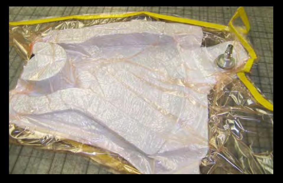
The vacuum valve should be positioned outside of the laminate with a breather connection to maintain vacuum flow.
