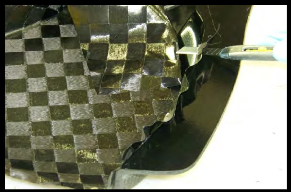
Cut away excessive material to allow consolidation at all corners. This helps in reducing the risk of bridging.
