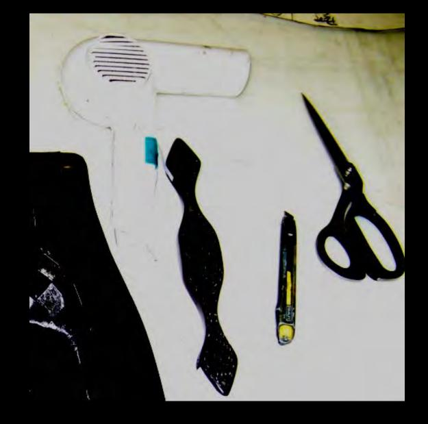
Tools to be used in this guide: Hairdryer, lamination tool, knife, scissors.
