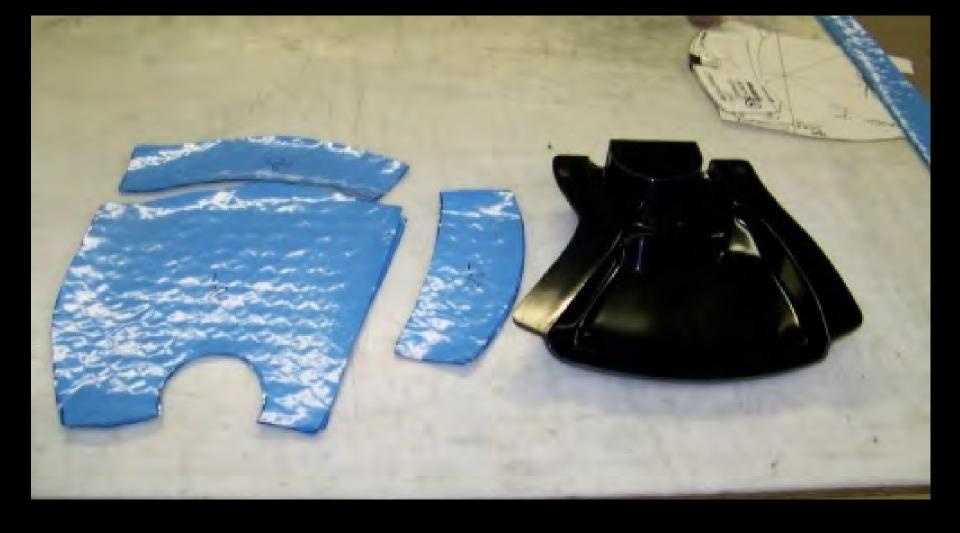
Use tool surfaces that are polished and release agents with relatively high degree of slip.
