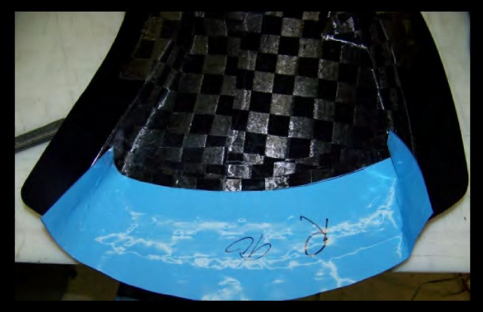
Stagger ply drop-offs at stiffened sections. There is no need to repeatedly debulk unless six layers or more are being used or otherwise recommended by prepreg manufacturer(s).
