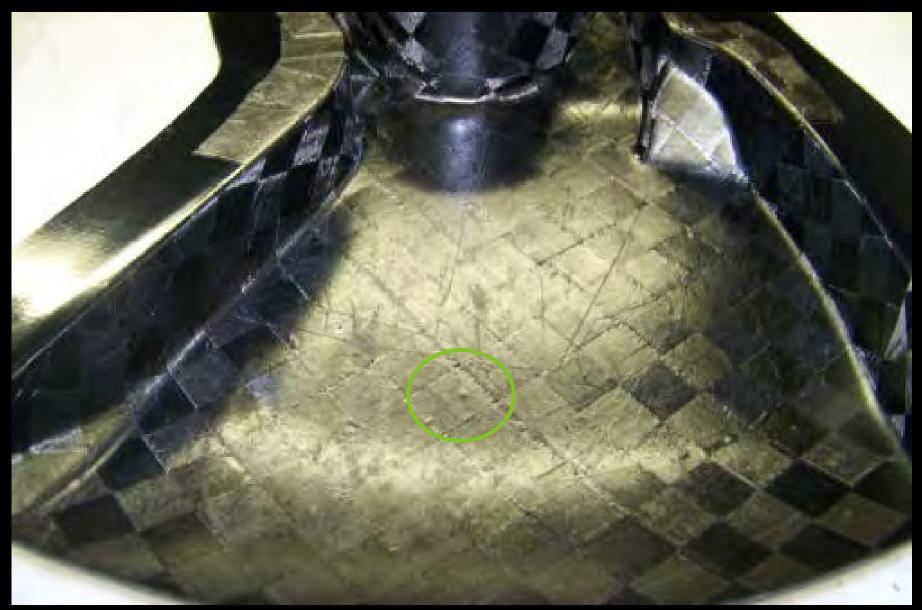
Vent possible bubbles to avoid trapping air at tool surface using needle or similar being careful not to scratch the mold surface.
