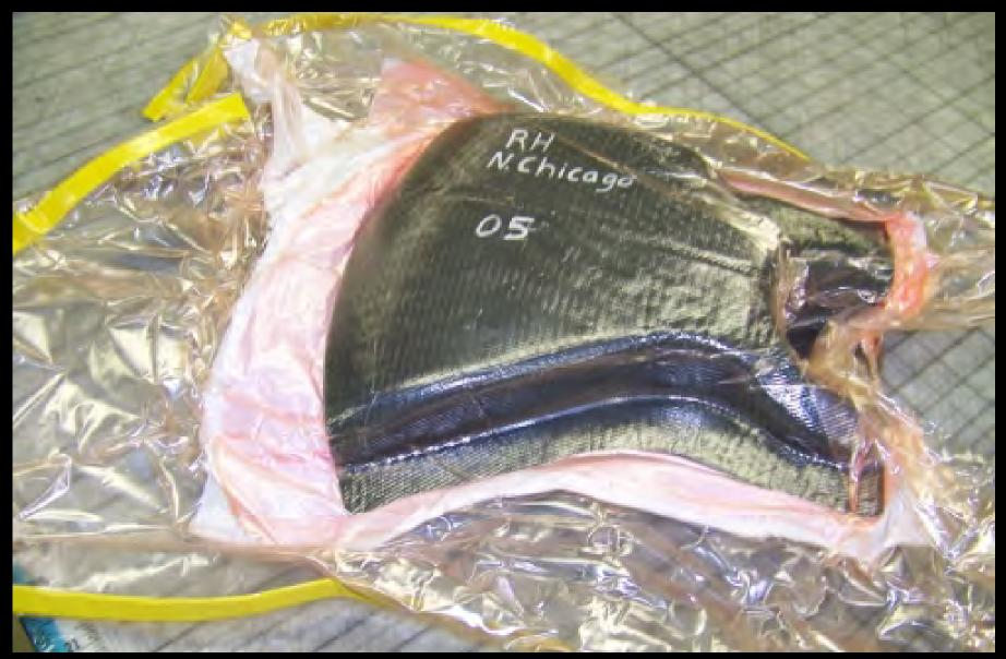
Envelope bag the tool when possible to avoid tool leakage leading to poor air evacuation.
