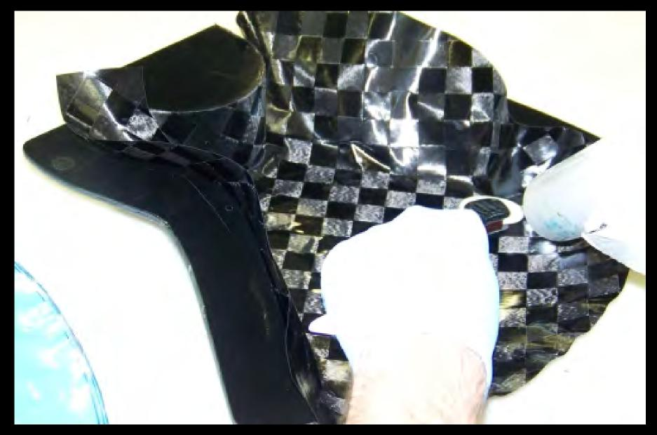
Work along 45-degree direction and soften the resin by using a hair dryer or heat gun to allow the fabric to scew.
