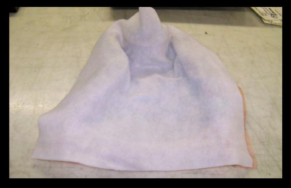
Follow standard bagging techniques. To maintain consistent vacuum pressure, the breather should cover the entire laminate.
