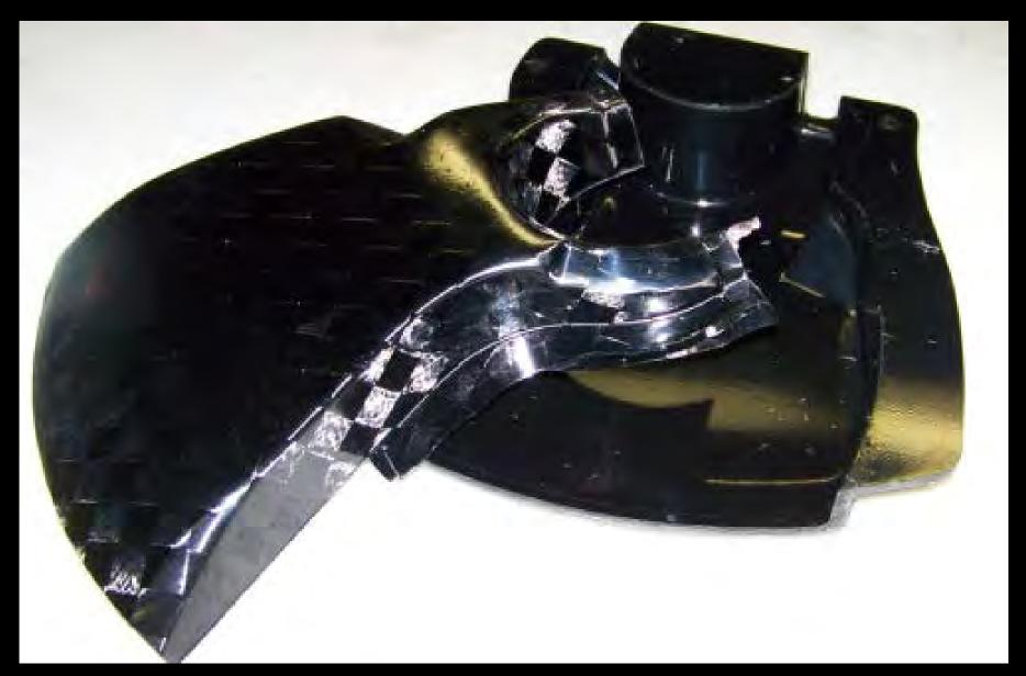
Demold the part. Notice well defined tight corners with no bridging on the relatively complex geometry of the finished part.
